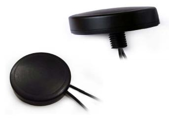
This low-profile antenna combines a GPS patch antenna with a +27dB filtered LNA and a multi-frequency antenna element capable of operating on all GSM frequencies 850/900/1800/1900/2100 Mhz
