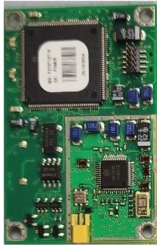
Motorola M12+ RF Dam PC trace around RF Section
