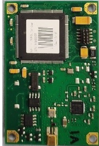
iLotus M12M No PC Trace around RF Section
