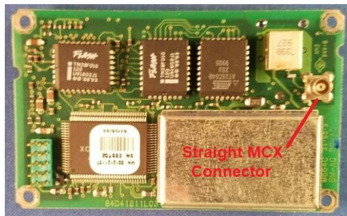
Motorola VP Oncore board with a straight (STR) MCX (UT+ is the same)
