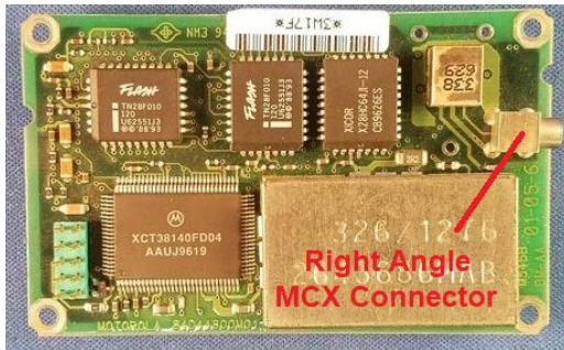
Motorola VP Oncore board with a right angle MCX (UT+ and GT+ are the same)
